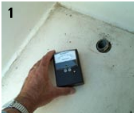
1. The moisture meter registered water saturation everywhere, so the entire cockpit sole would have to be opened up. 2. Using a diamond saw I cut the upper surface into strips for easy removal. 3. You can see how the water entered the core at the rudder post, progressing forward through the balsa core.
