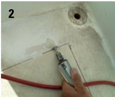
1. The moisture meter registered water saturation everywhere, so the entire cockpit sole would have to be opened up. 2. Using a diamond saw I cut the upper surface into strips for easy removal. 3. You can see how the water entered the core at the rudder post, progressing forward through the balsa core.
